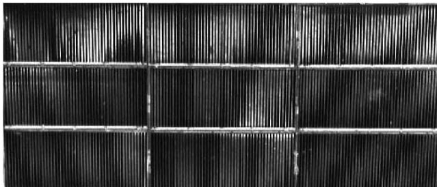
Fig. 2 Snapshot of the small sample used in arc plasma solar array experiments.
